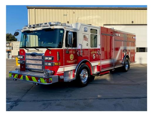
Another shot of our new Engine-5 on the ramp outside the "Blue Floor" at Pierce Manufacturing headquarters in Appleton, WI on March 15. The "Enforcer" style pumper has a 1500 GPM pump, 750-gallon water tank, and will be equipped as a "rescue-pumper" to handle fire rescue and suppression, emergency medical and special operation responses.
