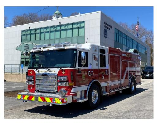
Our new Pierce Manufacturing Pumper designated Engine-5 shown here at City Hall shortly after being delivered on April 13. The truck is equipped with a 500 HP motor, 1,500 gallon per minute pump, and a 750 gallon water tank. the Fire Department personnel will undergo an extensive training program requiring several weeks., before the truck is placed in service.
