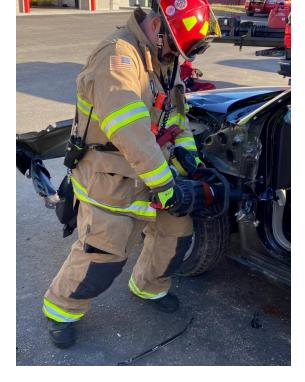
A-Shit Lt Drakopoulos evaluates a battery powered hydraulic cutter as part of the assessment process to purchase a set of battery powered hydraulic rescue tools through a FEMA Assistance to Firefighters Grant (AFG). The SFD extends appreciation to Chandler's Automotive and Towing of Sanford Me for donating, delivering, and picking up four junked vehicles used in the training and evaluation process.
